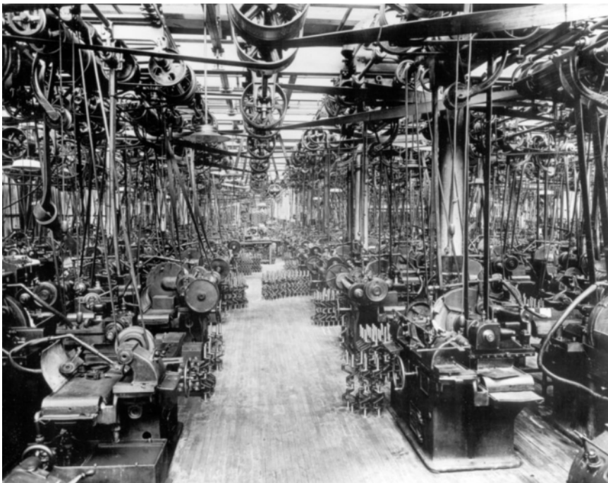
An example of the typical automotive machine shop early in the automotive age. There was a central power source, usually steam or water wheel. That power source turned overhead shafts to which were connected belts which powered each machine.
